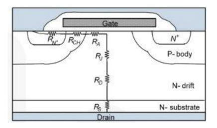
$R_{\mbox{\scriptsize ON}}$  is a product of the cumulative resistances from the drain to the source of a MOSFET device.
